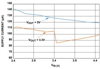
FIGURE 7. SUPPLY CURRENT vs VIN
