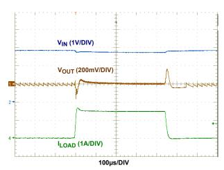
FIGURE 11. LOAD STEP RESPONSE,  $V_{IN}$  = 2.7V,  $I_{LOAD}$  = 10mA -> 1500mA -> 10mA
