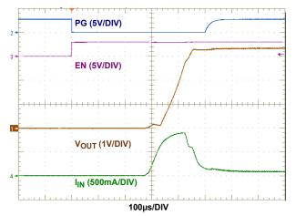
FIGURE 10. START-UP WAVEFORM  $50\Omega$  LOAD,  $V_{\mbox{\footnotesize{IN}}}$  = 3V,  $V_{\mbox{\footnotesize{OUT}}}$  = 3.3V
