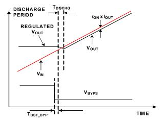
FIGURE 21. FORCED MODE, BOOST TO BYPASS
