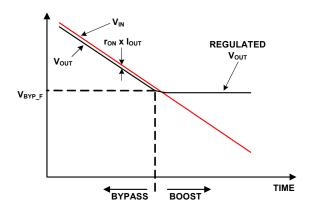
FIGURE 18. AUTO BYPASS WITH FALLING VIN
