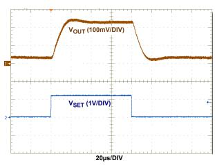
FIGURE 13.  $V_{SET}$  TOGGLE RESPONSE,  $V_{IN}$  = 3V,  $V_{OUT}$  = 3.3V, LOAD = 0.5A
