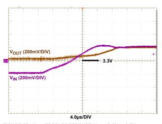
FIGURE 15.  $V_{SET}$  TOGGLE RESPONSE,  $V_{IN}$  = 3.1V -> 3.5V, LOAD = 1A
