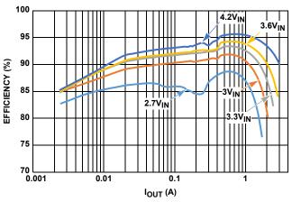
FIGURE 6. EFFICIENCY vs LOAD CURRENT, V<sub>OUT</sub> = 5V
