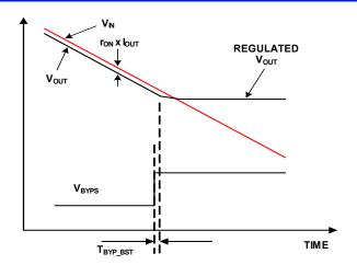
FIGURE 20. FORCED MODE, BYPASS TO BOOST
