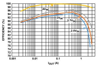
FIGURE 2. EFFICIENCY vs LOAD CURRENT, V<sub>OUT</sub> = 3.3V
