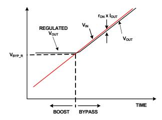
FIGURE 19. AUTO BYPASS WITH RISING  $V_{\mbox{\scriptsize IN}}$
