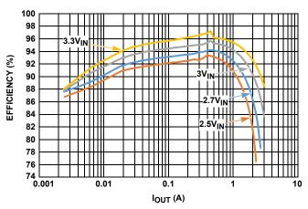
FIGURE 5. EFFICIENCY vs LOAD CURRENT, V<sub>OUT</sub> = 3.5V
