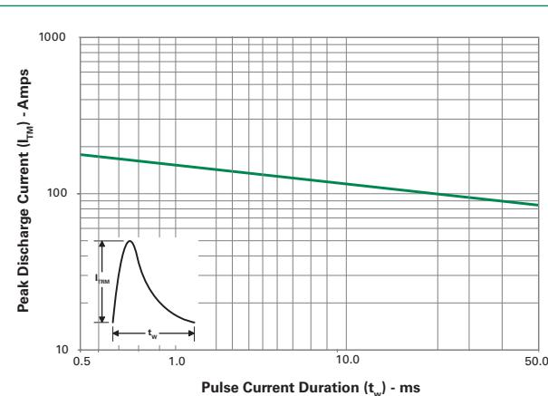
**Figure 12: Peak Capacitor Discharge Current Derating**
