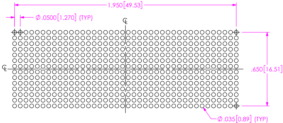
RECOMMENDED STENCIL LAYOUT ALL DIMENSIONS ARE SYMMETRIC ABOUT THE CENTERLINE STENCIL TO BE .0060 [0.157] THICK
