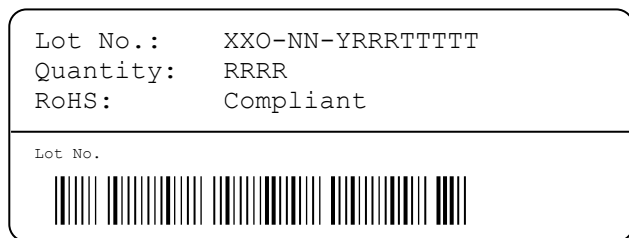
Figure 14: First label on reel: XX = Sensor Type (21 for SHT21), O = Output mode (D = Digital, P = PWM, S = SDM), NN = product revision no., Y = last digit of year, RRR = number of sensors on reel divided by 10 (200 for 2000 units), TTTTT = Traceability Code.
