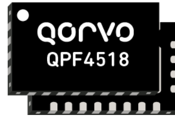
24 Pin 5x3 mm QFN Package
