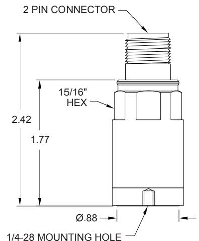
Notes: <sup>1</sup> For a 100 mV/ips sensor with  $\pm 5\%$  sensitivity tolerance, order model 793V100-5.
