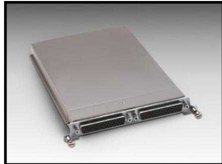
The Model 7703 plug-in module offers 32 channels of 2-pole or 16 channels of 4-pole multiplexer switching that can be configured as two independent banks of multiplexers. The non-latching reed relays provide high speeds and are designed for 300 volt, 500mA; 10VA. The relay closures are stored in onboard memory. The Model 7703 is ideal for RTD and thermistor temperature applications.
