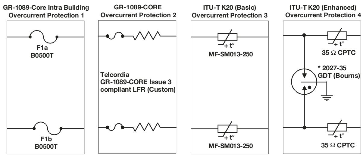
Figure 5. Typical Overcurrent Protection
