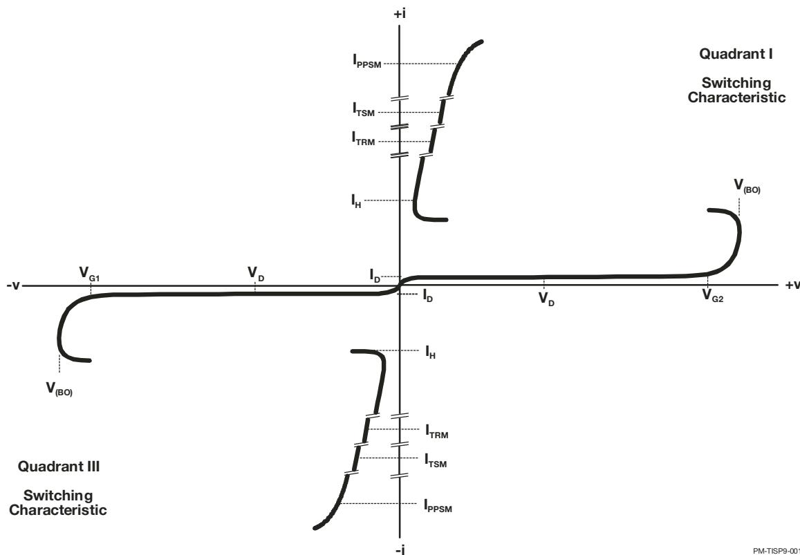
**Figure 1. Voltage-Current Characteristic**
