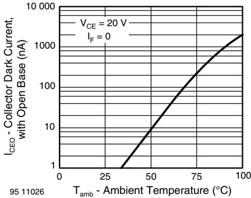
Fig. 7 - Collector Dark Current vs. Ambient Temperature
