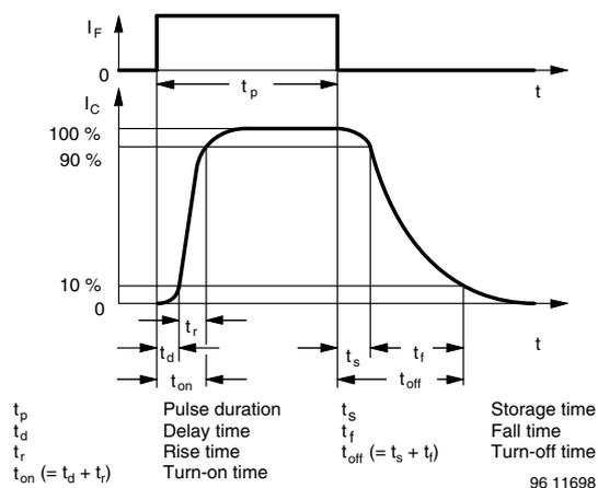
Fig. 3 - Switching Times
