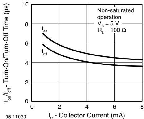
Fig. 13 - Turn-on/off Time vs. Collector Current
