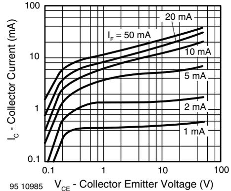
Fig. 9 - Collector Current vs. Collector Emitter Voltage
