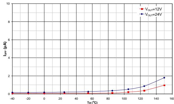
**8.8  $I_{OFF}$  vs.  $V_{OUT}$**
