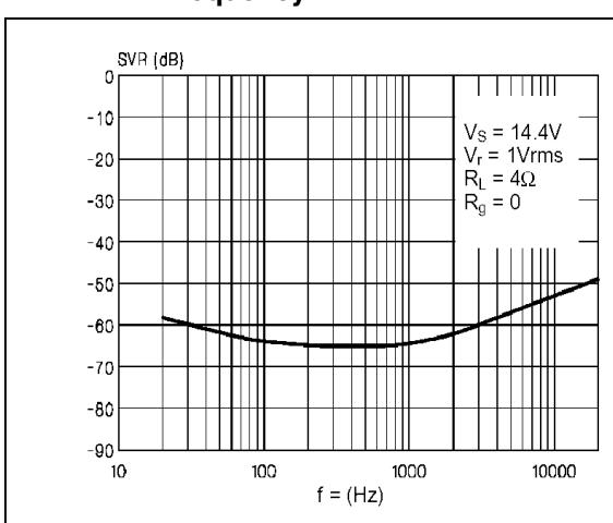
**Figure 11. Common mode rejection vs. frequency**
