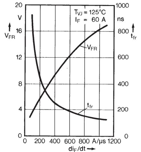
Fig. 6 Peak forward voltage versus  $di_F/dt$ .
