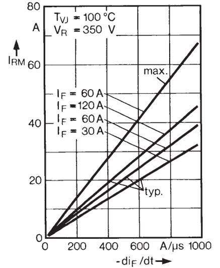
Fig. 3 Peak reverse current versus  $-di_F/dt$ .
