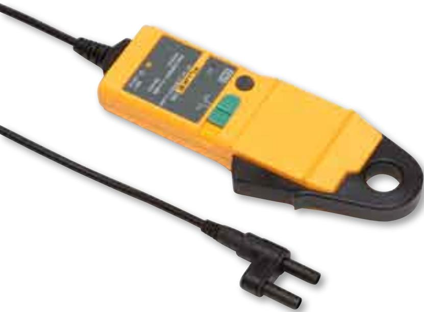
The i30 current clamp is based on Hall effect technology for use in measurement of both dc and ac current. The i30 may be used in conjunction with multimeters, recorders and other suitable recording instruments for accurate non-intrusive current measurement.
