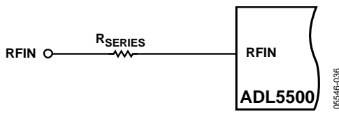
Figure 36. Attenuating the Input Signal
