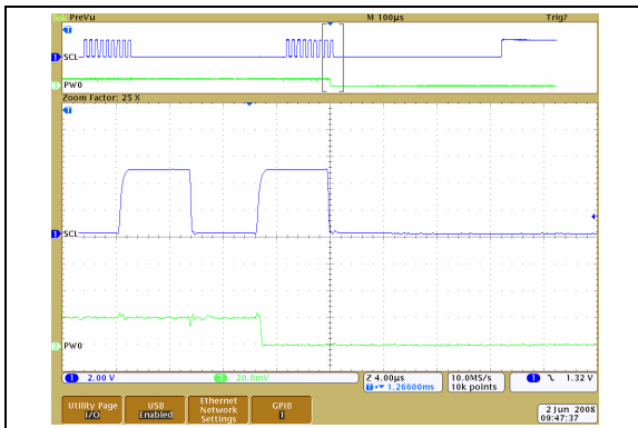
FIGURE 2-83: 100\text{ k}\Omega – Low-Voltage Decrement Wiper Settling Time ( V_{DD} = 5.5\text{V} ) ( 1\ \mu\text{s}/\text{Div} ).
