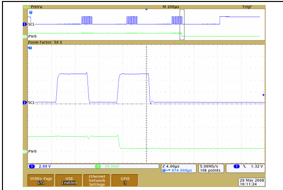
FIGURE 2-62: 50\text{ k}\Omega – Low-Voltage Decrement Wiper Settling Time ( V_{DD} = 2.7\text{V} ) ( 1\ \mu\text{s}/\text{Div} ).
