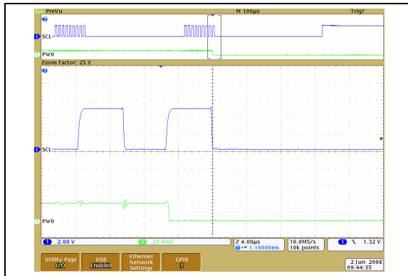
FIGURE 2-82: 100 k \Omega – Low-Voltage Decrement Wiper Settling Time ( V_{DD} = 2.7\text{V} ) (1 \mu\text{s}/\text{Div} ).
