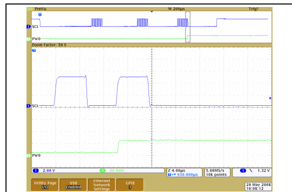
FIGURE 2-65: 50\text{ k}\Omega – Low-Voltage Increment Wiper Settling Time ( V_{DD} = 5.5\text{V} ) ( 1\text{ }\mu\text{s/Div} ).
