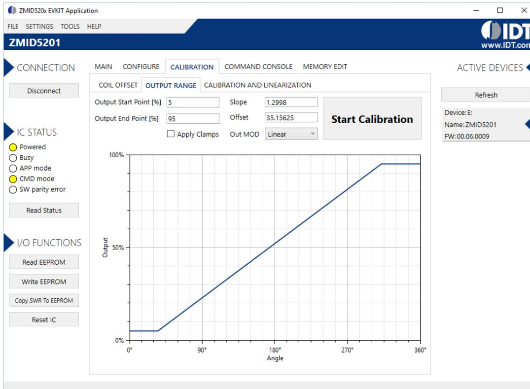
There are four values that can be edited on the “OUTPUT RANGE” sub-tab for subsequent use during the calibration procedure:
