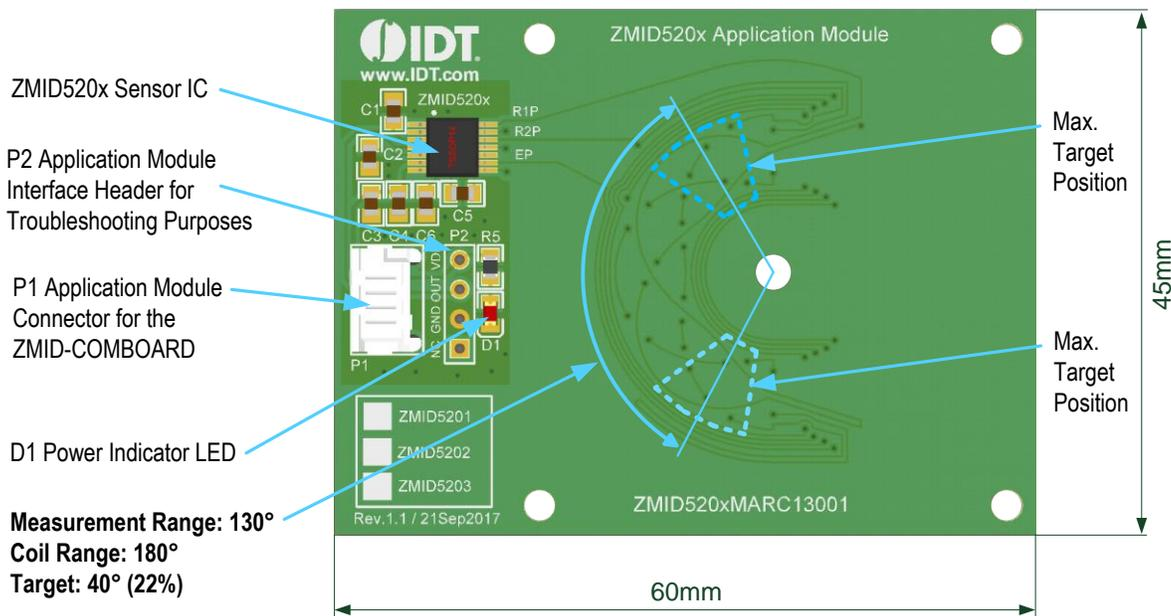
**Figure 6. ZMID520x Linear Application Module – Overview**
