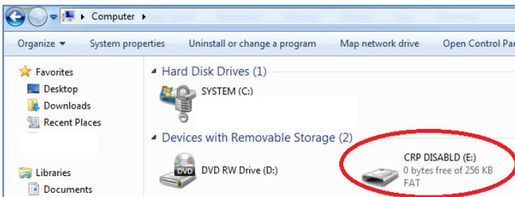
6. Delete the “firmware.bin” file from the device. Recommendation: Store a copy of the file on the user’s computer as a backup.
