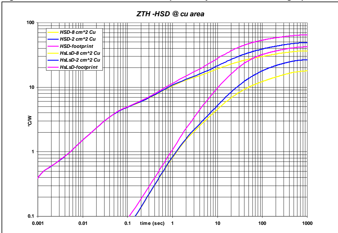
Figure 20. PowerSSO-36 LSD thermal impedance junction ambient single pulse
