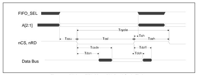
Figure 6.3 RX Data FIFO Direct PIO Read Cycle Timing
