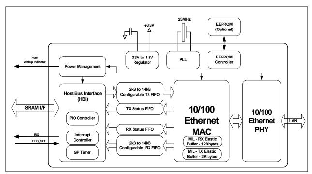
Figure 1.2 Internal Block Diagram
