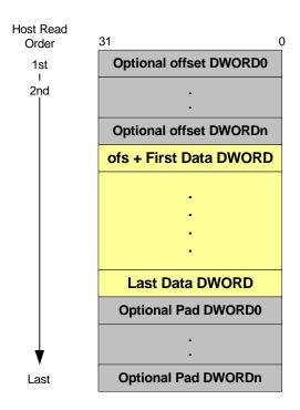
Figure 3.17 RX Packet Format
