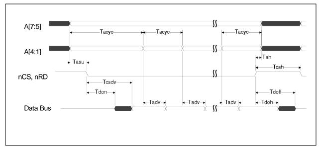
Figure 6.2 PIO Burst Read Cycle Timing
