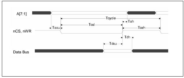
Figure 6.5 PIO Write Cycle Timing
