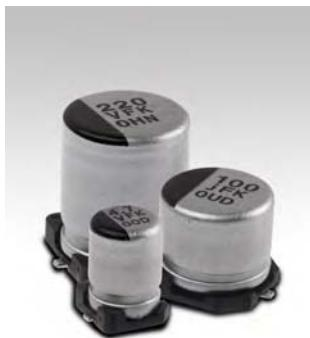
Type AVEZ Capacitors are rated for 1000 hours at 105 °C with low impedance characteristics. They are ideal for high density PC board packaging. The Type AVEZ offers a low in-place-cost for a high quality performer. The vertical cylindrical cases facilitate automatic mounting and reflow soldering into the same footprint of like-rated tantalum capacitors except without the need for voltage derating. Type AVEZ is RoHS compliant.
