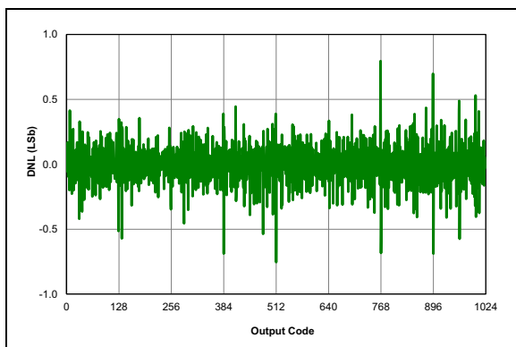
FIGURE 31-77: ADC 10-bit Mode, Single-Ended DNL, V_{DD} = 3.0V , T_{AD} = 1\ \mu S , 25^\circ C .
