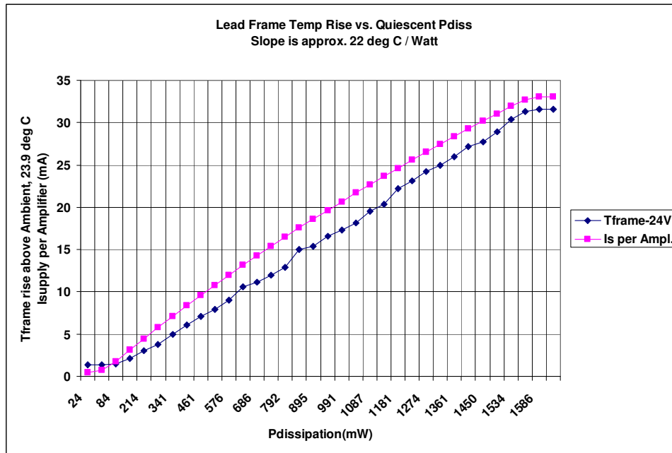
Figure 7. Temperature Rise and Supply Current as Quiescent Power Dissipation is Increased (Vcc = 24Vdc).
