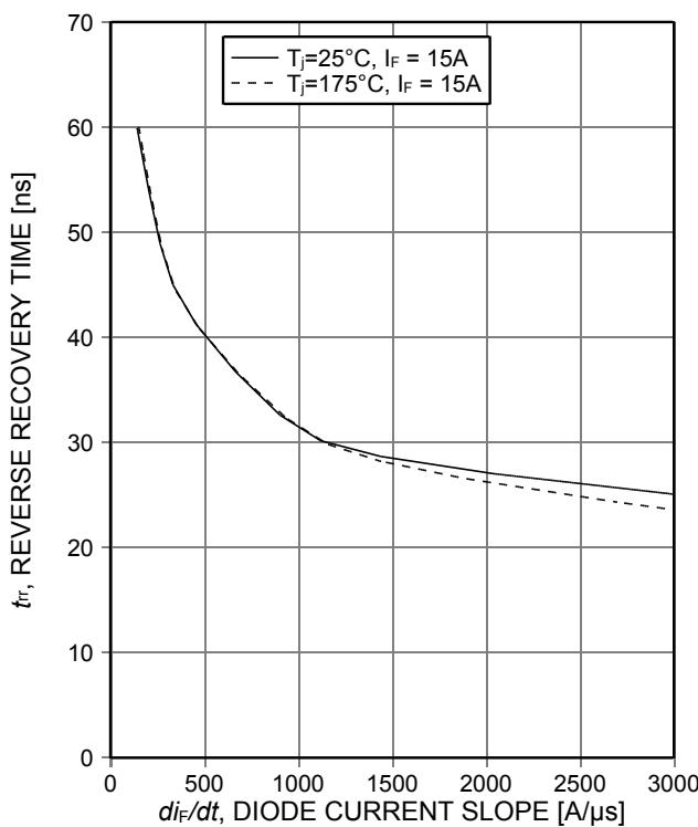
Figure 3. Typical reverse recovery time as a function of diode current slope
