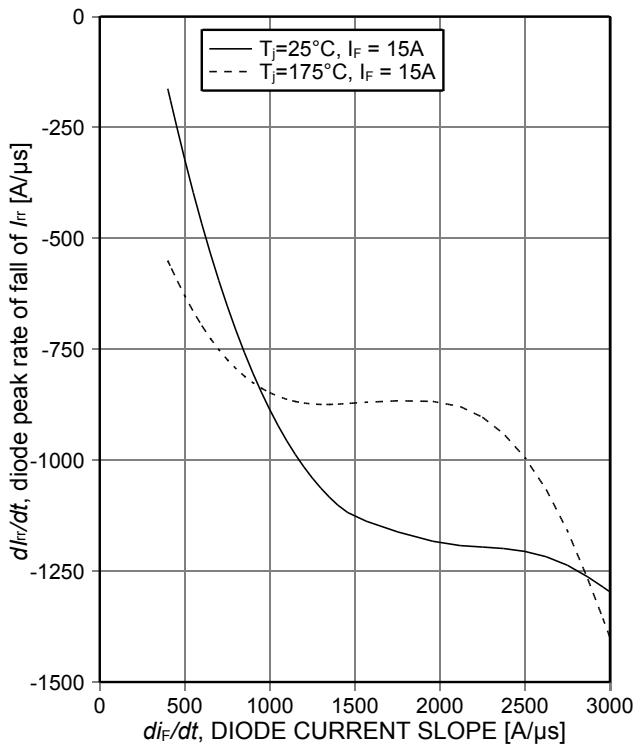
Figure 6. Typical diode peak rate of fall of rev. rec. current per diode as a function of diode current slope ( $V_R=400\text{V}$ )
