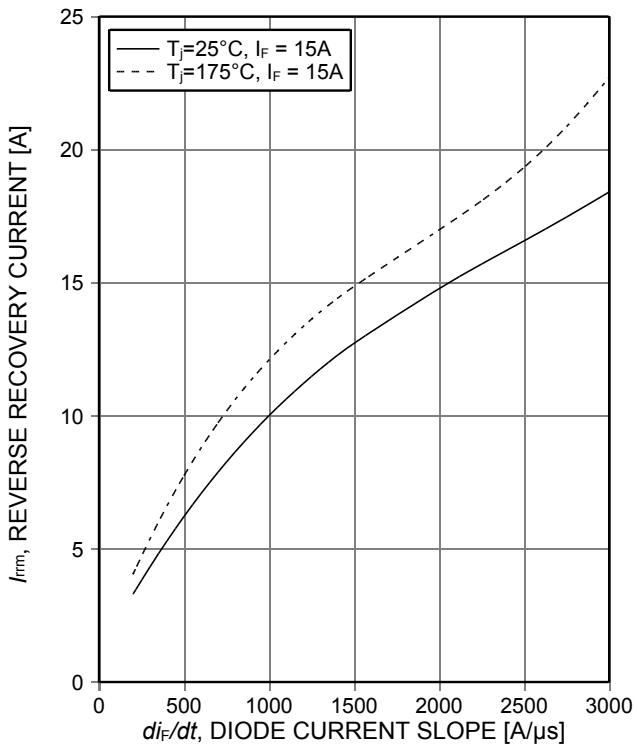
Figure 5. Typical peak reverse recovery current per diode as a function of diode current slope ( $V_R=400\text{V}$ )
