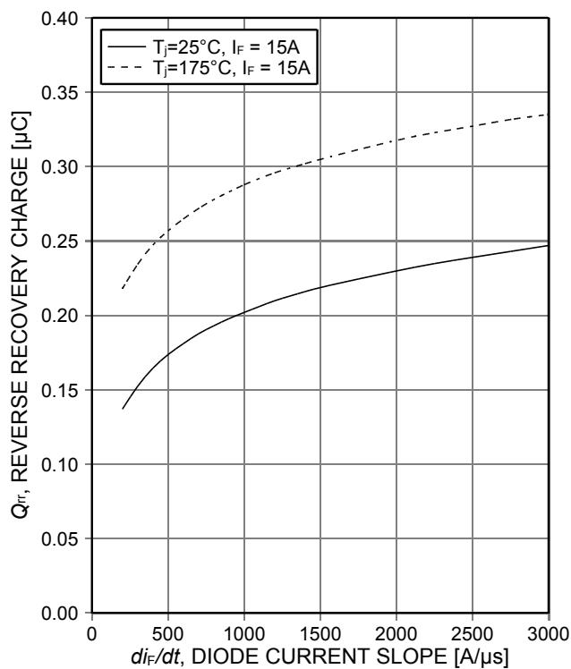
Figure 4. Typical reverse recovery charge per diode as a function of diode current slope
