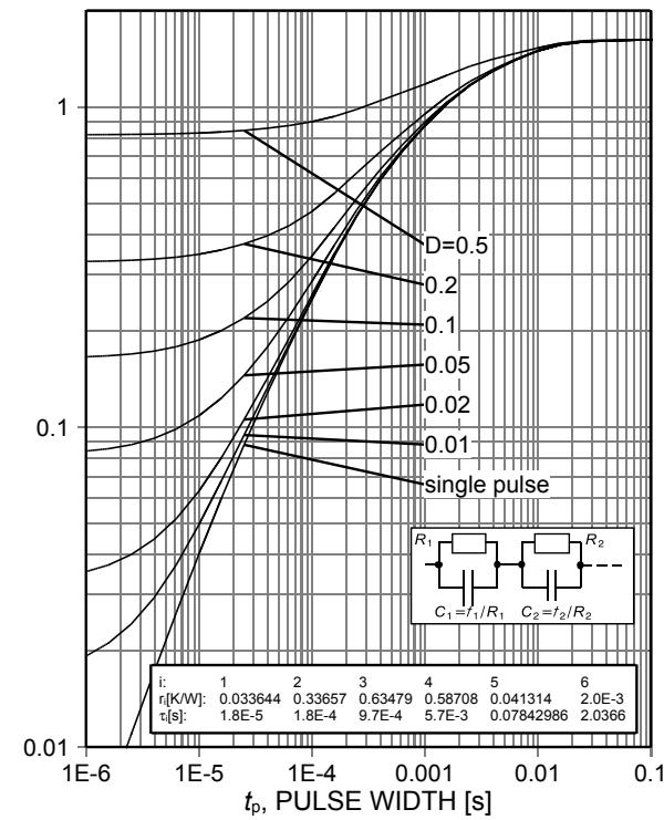
Figure 2. Diode transient thermal impedance per diode as a function of pulse width
