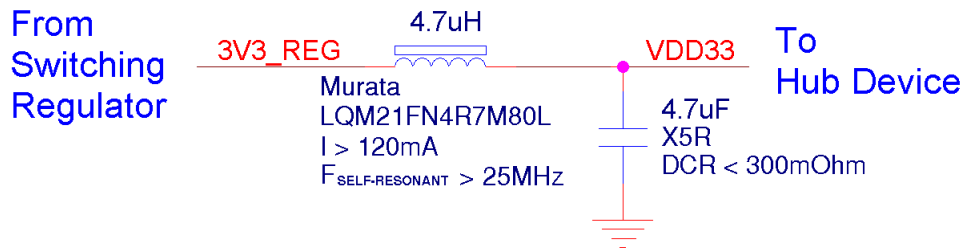
Figure 2.2 Example Switching Regulator Noise Filter
