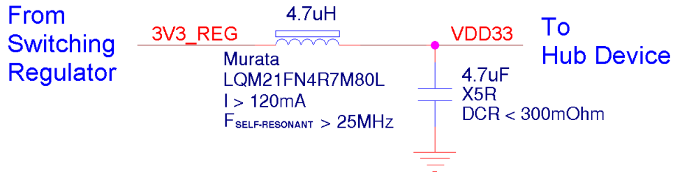
Figure 2.2 Example Switching Regulator Noise Filter
