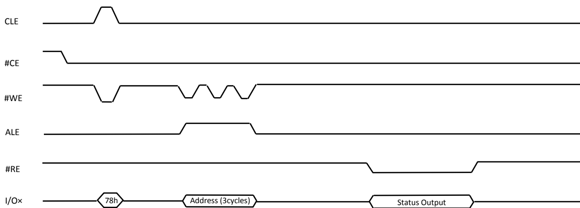
Figure 9-10 Read Status Enhanced (78h) Operation
