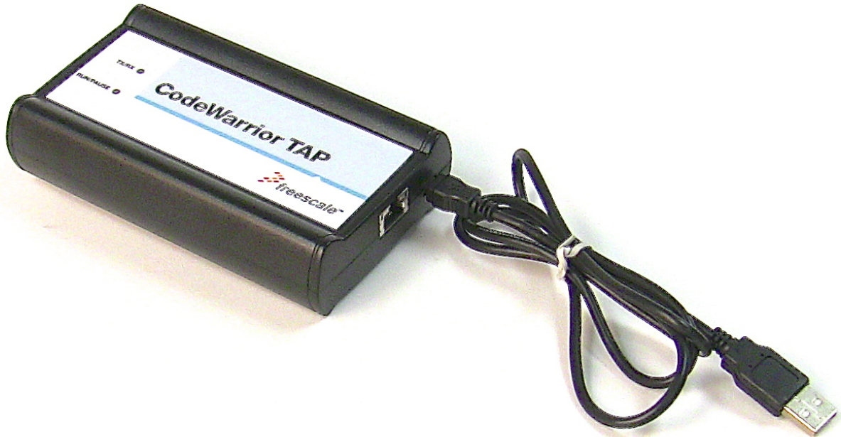
Figure 5. CodeWarrior TAP probe with USB cable attached
