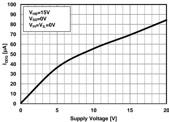
Figure 9.  $I_{DDQ}$  vs. Supply Voltage( $V_{DD}$ )
