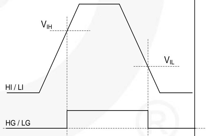
**Figure 63. PWM threshold definitions**
