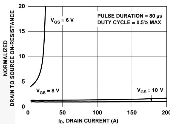
Figure 51. Normalized On-Resistance vs. Drain Current and Gate Voltage
