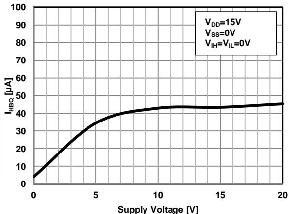
Figure 11. .  $I_{HBQ}$  vs. Supply Voltage( $V_{DD}$ )
