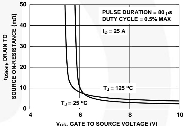
Figure 41. On-Resistance vs. Gate to Source Voltage
