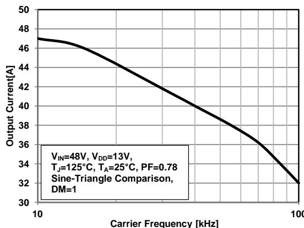
Figure 37. Output Current Vs. Carrier or Modulation Frequency
