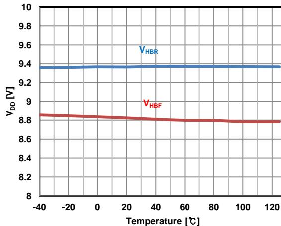
Figure 30.  $V_{HB}$  UVLO Threshold Voltage vs. Temp.
