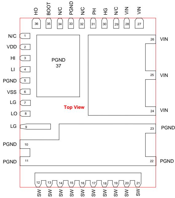
Figure 2. Pin Configuration (6.0mm x 7.5mm Package)
