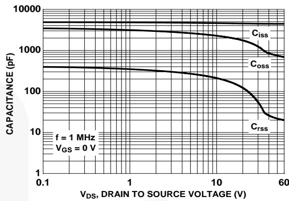
Figure 57. Capacitance vs. Drain to Source Voltage
