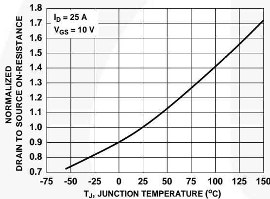
Figure 52. Normalized On Resistance vs. Junction Temperature
