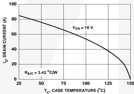
Figure 46. Maximum Continuous Drain Current vs. Case Temperature
