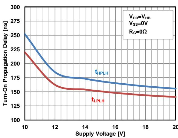
Figure 13. Turn-On Propagation Delay vs. Supply Voltage( $V_{DD}$ )
