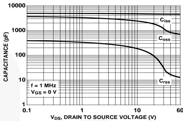
Figure 45. Capacitance vs. Drain to Source Voltage
