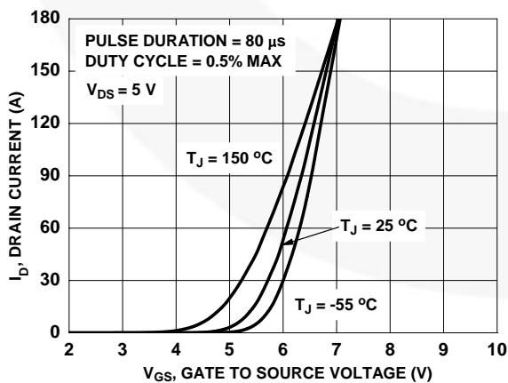
Figure 42. Transfer Characteristics
