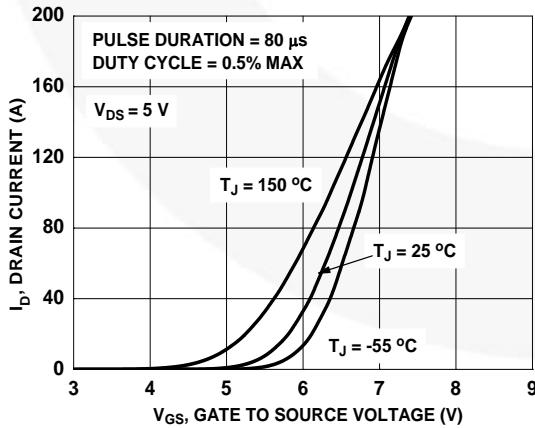
Figure 54. Transfer Characteristics
