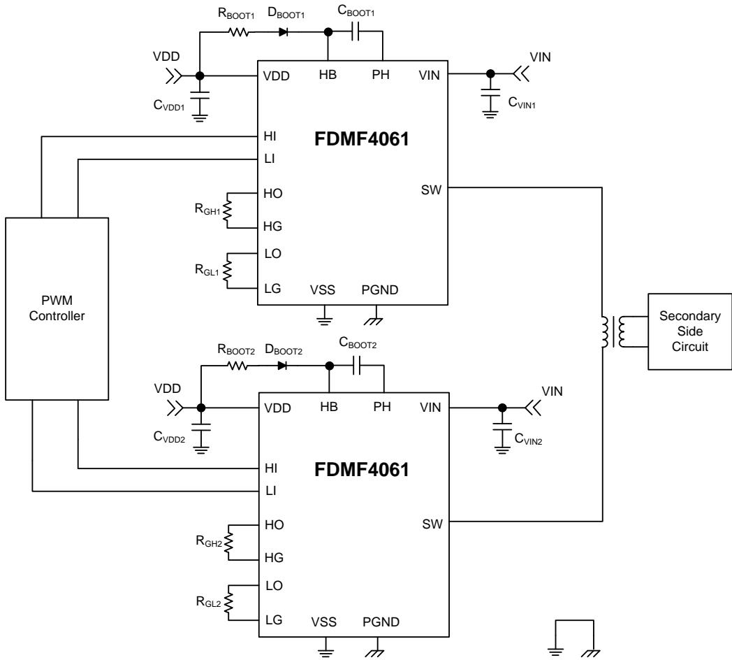
**Figure 8. Full-Bridge Converter**
