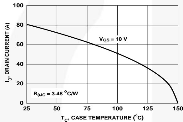
Figure 58. Maximum Continuous Drain Current vs. Case Temperature
