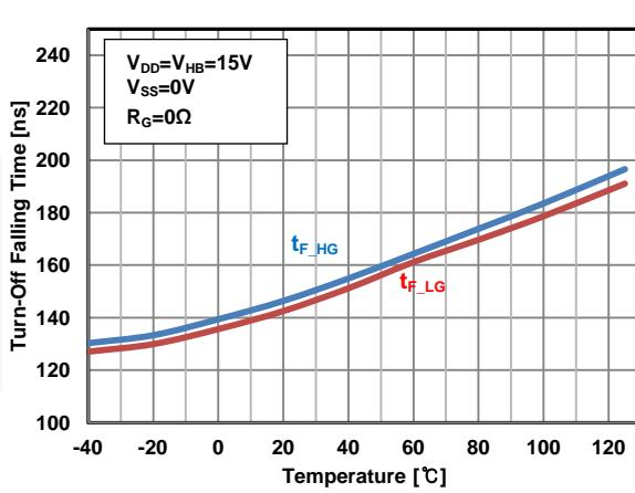
Figure 20. Turn-Off Falling Time vs. Temp.
