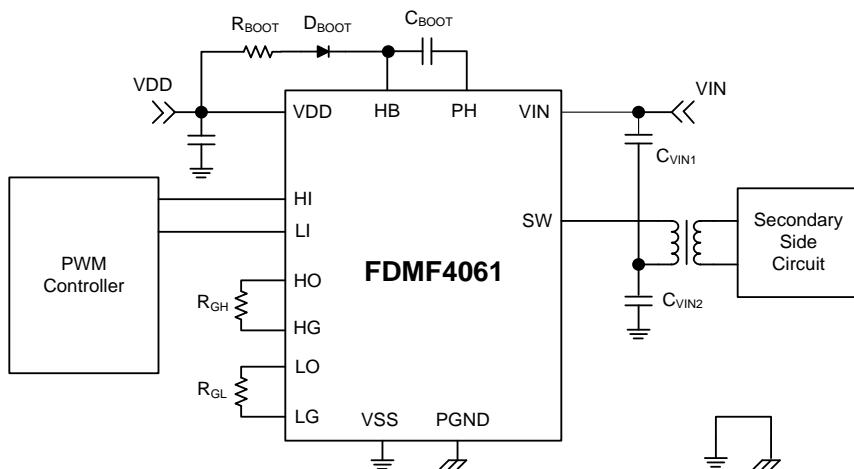
Figure 7. Half-Bridge Converter
