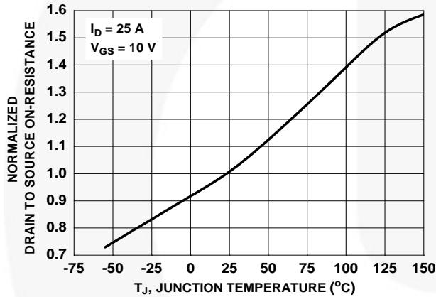
Figure 40. Normalized On Resistance vs. Junction Temperature
