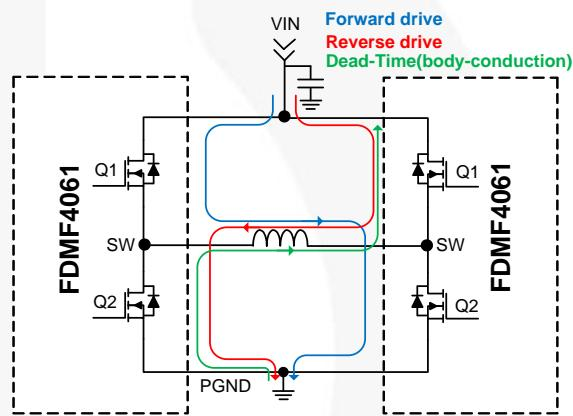
Figure 65. H-bridge motor drive
