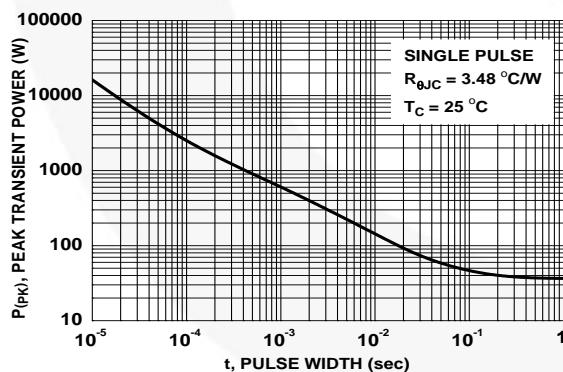
Figure 48. Single Pulse Maximum Power Dissipation
