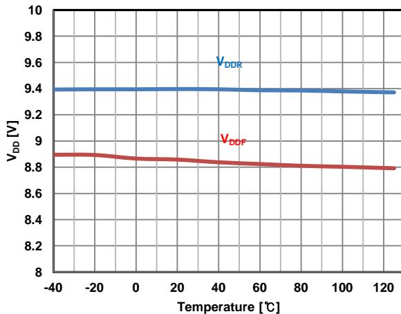
Figure 29.  $V_{DD}$  UVLO Threshold Voltage vs. Temp.
