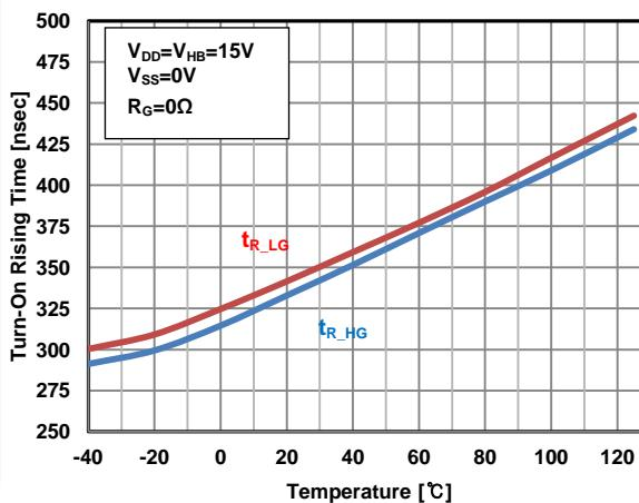
Figure 18. Turn-On Rising Time vs. Temp.
