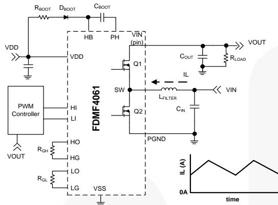
**Figure 67. Synchronous Boost Converter operating in CCM**
