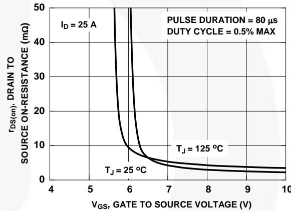
Figure 53. On-Resistance vs. Gate to Source Voltage
