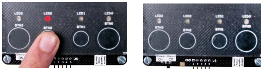
Figure 3-11. Kit with Delay Off Feature Disabled
