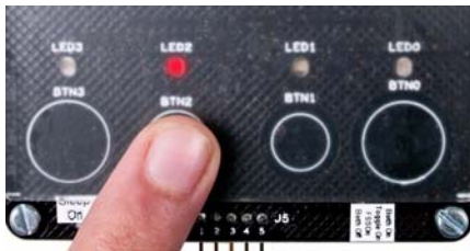
1. Touch a button; LED turns on
