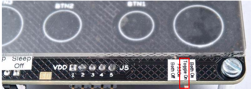
Figure 3-3. Switch Position for Toggle Feature
