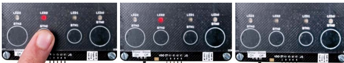
Figure 3-13. Test Sequence for Delay Off Feature
