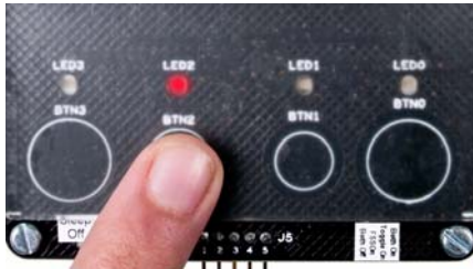
1. Touch a button; LED turns on
