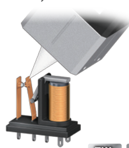
Operation inspection of relay contacts
