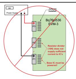
Figure 3. Incorrect Connections, Base IC Not Powered
