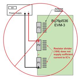
Figure 5. Incorrect Connections, Top IC Not Powered, IC1,2 Insufficient V<sub>BAT</sub>
