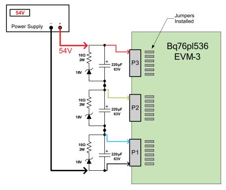
Figure 2. Alternate Connection for Single 54V Supply
