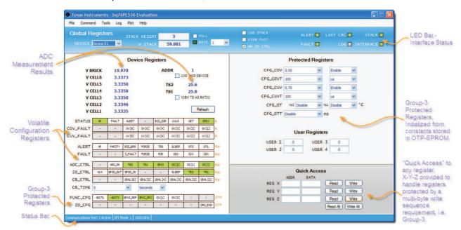
VBRIC K The voltage measured by the bq76PL536 between the BATx and VSS pins
