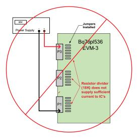
Figure 4. Incorrect Connections, Insufficient V<sub>BAT</sub> Per IC
