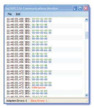
Figure 7. SPI Monitor Showing Communications Error
