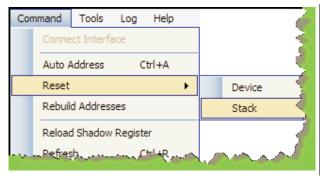
Because the part is shipped unprogrammed, the result of reloading the shadow registers is to transfer all zeros to the shadow cells, and will usually result in many ALERTS and FAULTS being triggered which are normally hidden by the GUI per the OPTION menu settings (see below).
