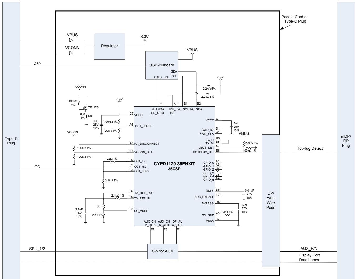
**Figure 7. Type-C to DisplayPort/mini-DisplayPort Application Using 40-QFN Package**
