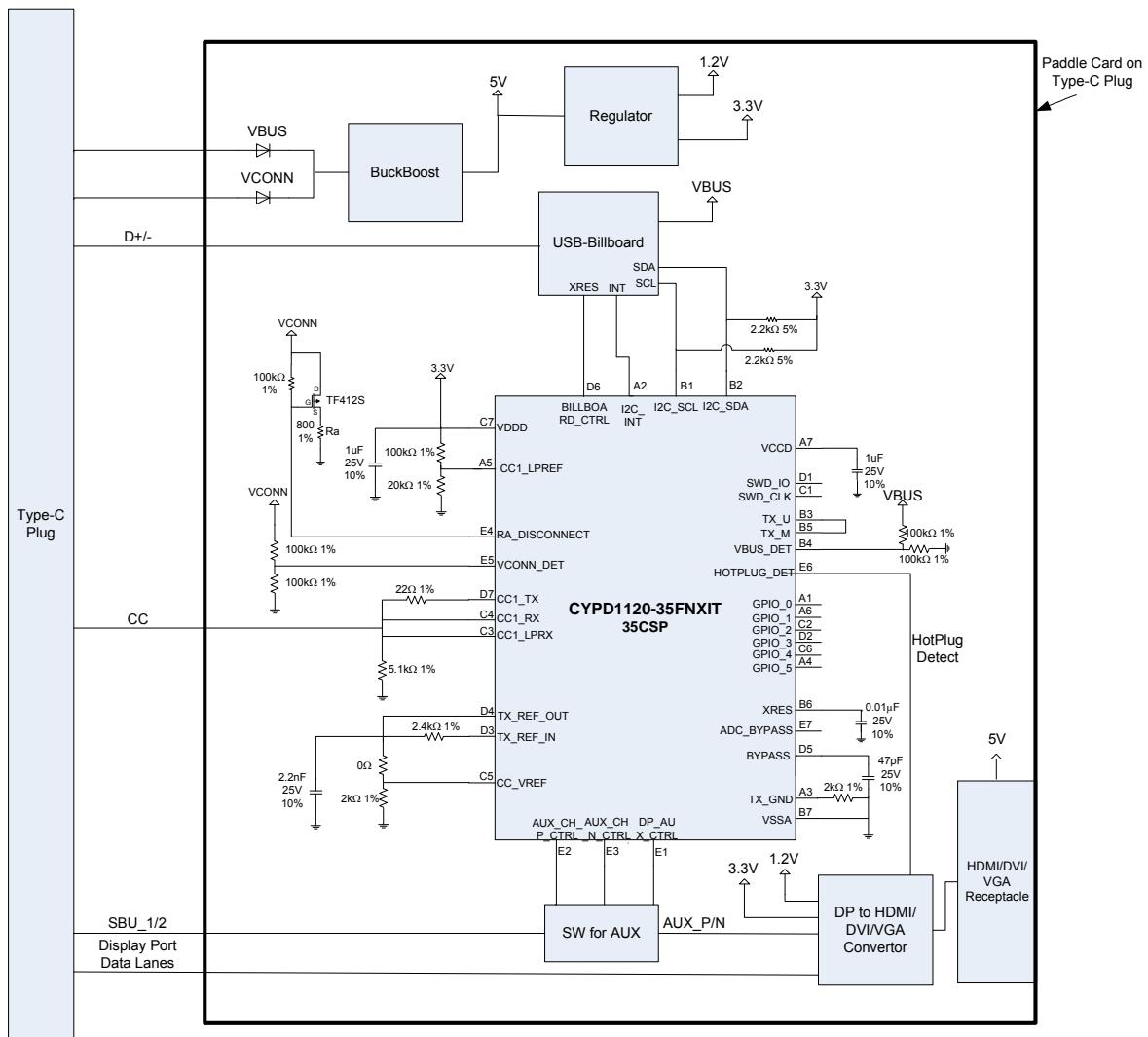
**Figure 9. Type-C to HDMI Application Using 40-QFN Package**
