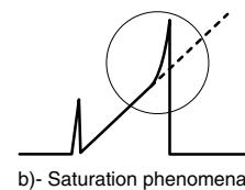
(3)In this case, there is possibility that a breakdown may occur due to surpassing the rated current of the switch it is necessary to have over current protection circuit or modify transformer design.
