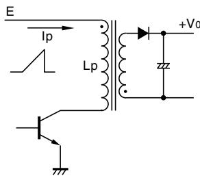
$$\text{Energy stored in the inductor } L_p \text{ is } W = \frac{1}{2} \times L_p \times I_p^2 \times [J]$$
