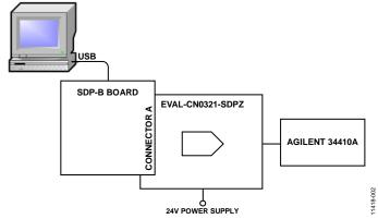
Figure 2. Test Setup Functional Diagram
