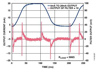
Figure 7. Analog Rate of Change Waveform
