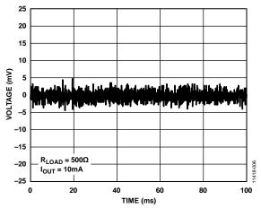
Figure 6. Output Noise During Silence Waveform
