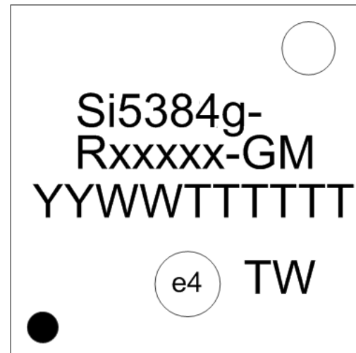
Figure 12.2. Si5384 Top Marking
