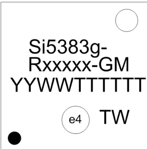
Figure 12.1. Si5383 Top Marking
