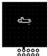
a. 53^{\circ}\text{C}/\text{W} when mounted on a 1\text{ in}^2 pad of 2 oz copper
