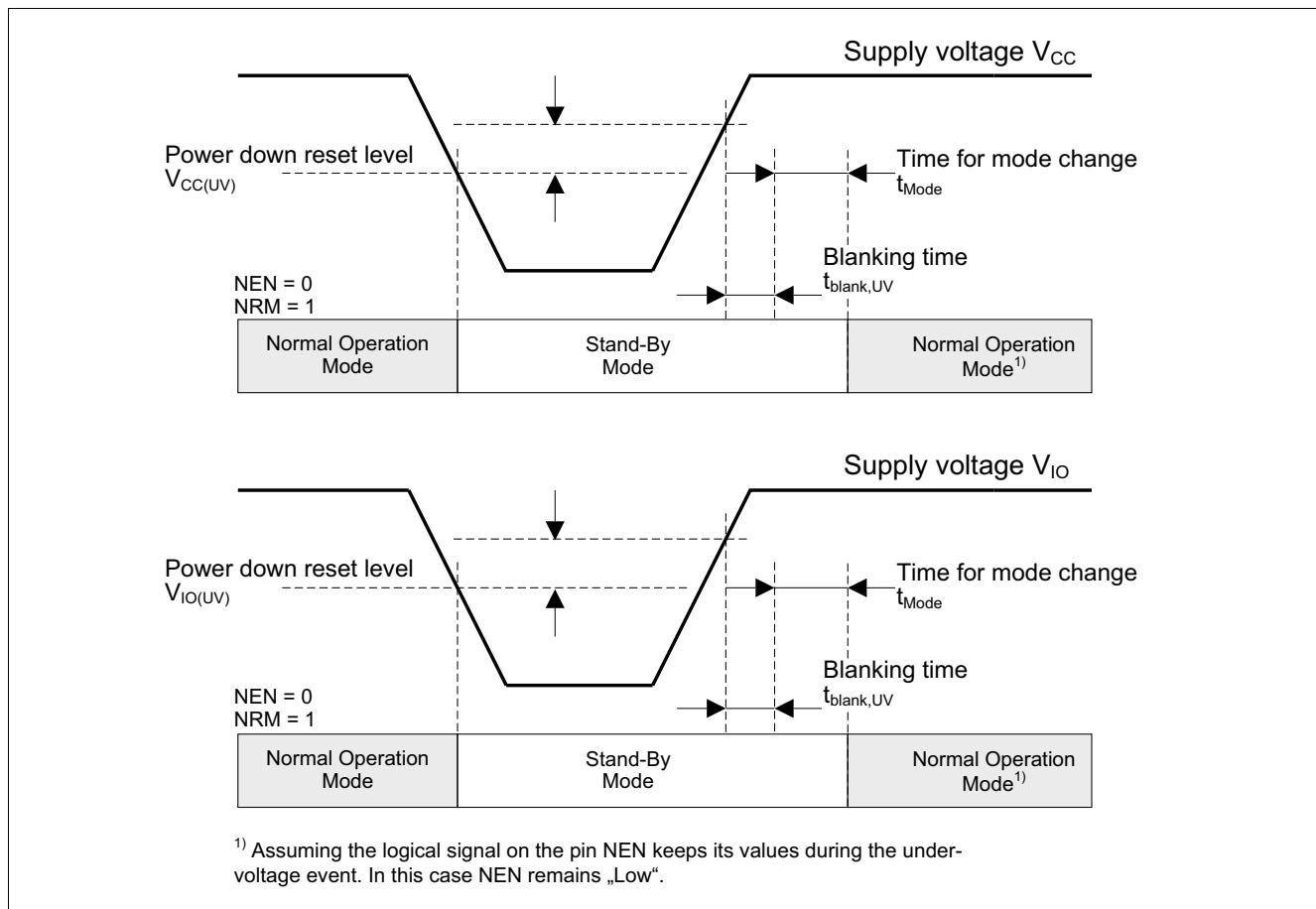
**Figure 6** Under-Voltage detection on  $V_{CC}$  and  $V_{IO}$
