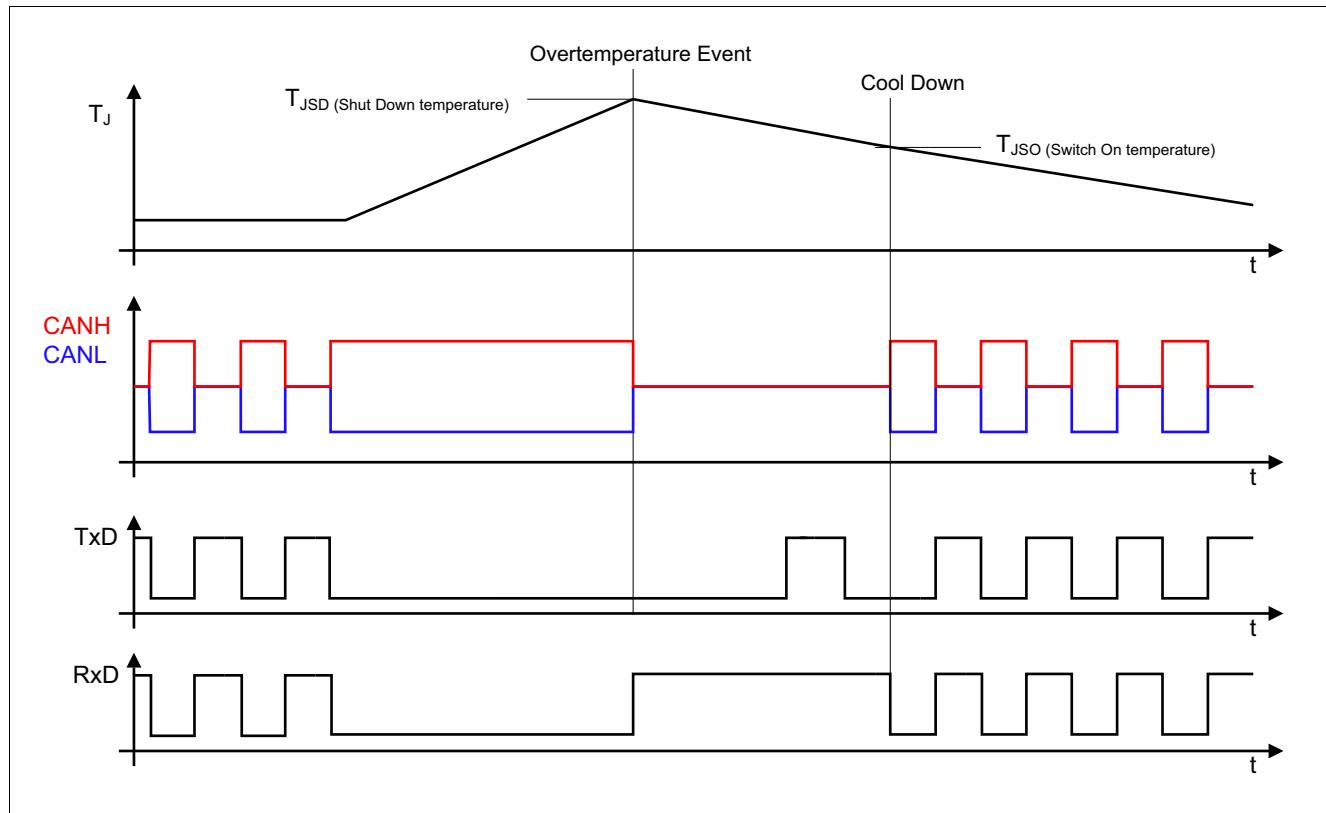
Figure 7 Over-Temperature protection
