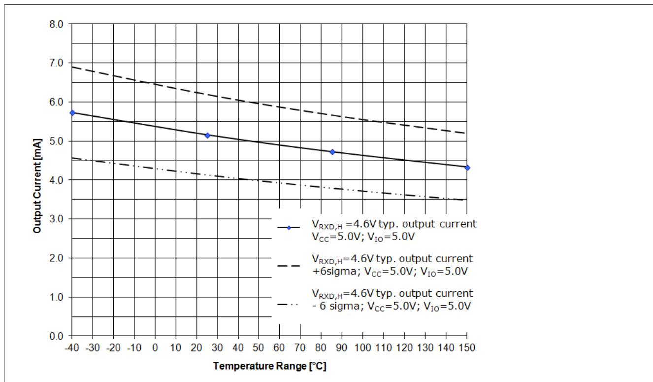
**Figure 11** RxD Output driver capability for a logical “High” signal  $V_{RXD,H}=4.6 \text{ V}$ ,  $V_{CC}=5.0 \text{ V}$ ,  $V_{IO}=5.0 \text{ V}$ <sup>1)</sup>
