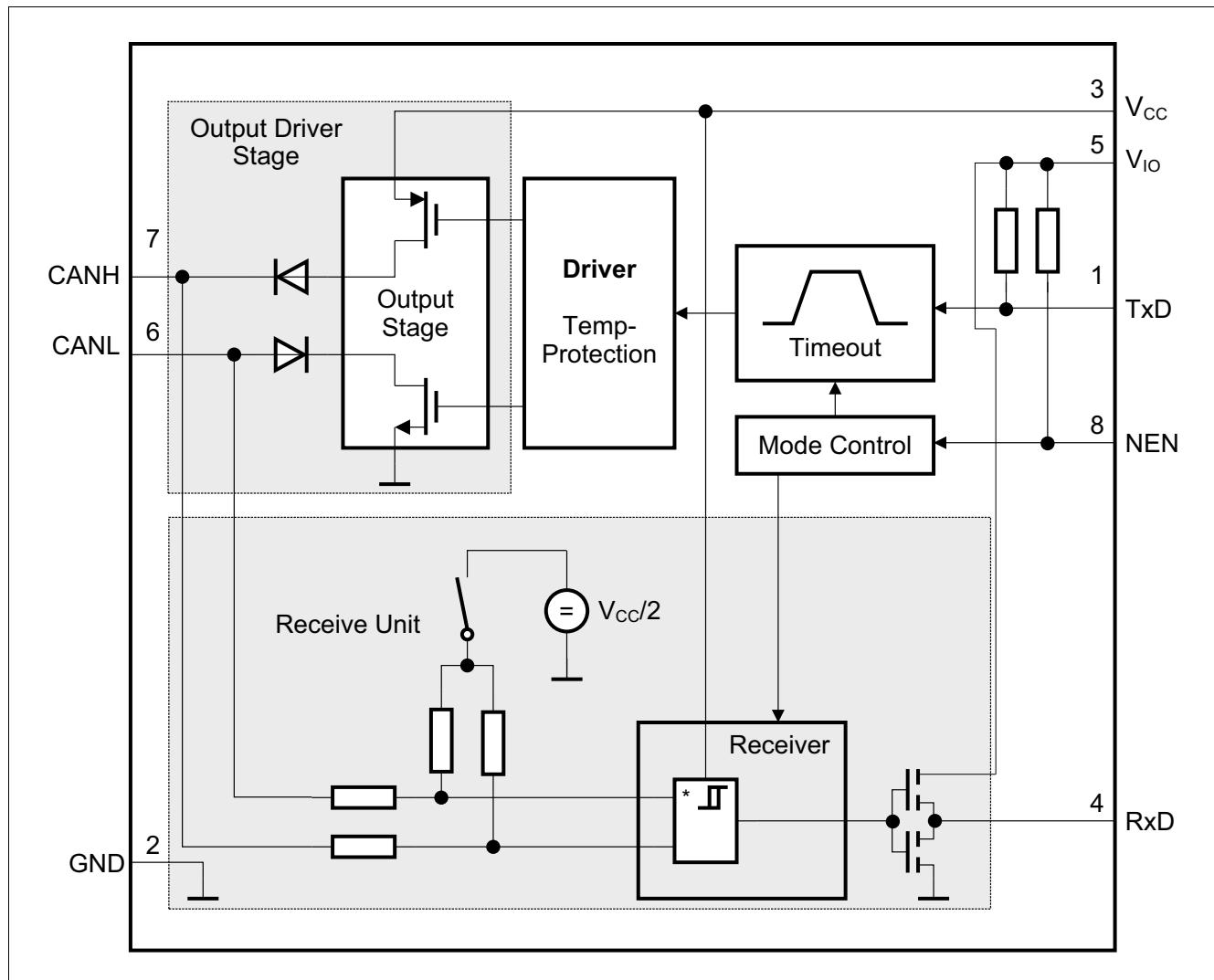
Figure 1 Block Diagram
