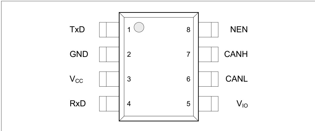
Figure 2 Pin Configuration
