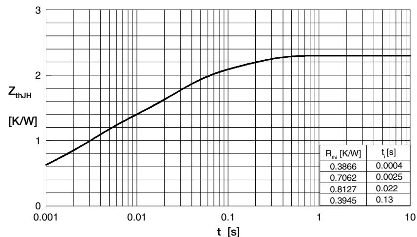
Fig. 8 Transient thermal resistance junction to case  $Z_{thJH}$
