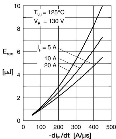
Fig. 7 Typ. recovery energy  $E_{rec}$  versus  $-di_F/dt$
