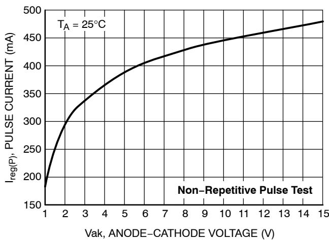
**Figure 3. Pulse Current (I<sub>reg(P)</sub>) vs. Anode-Cathode Voltage (Vak)**
