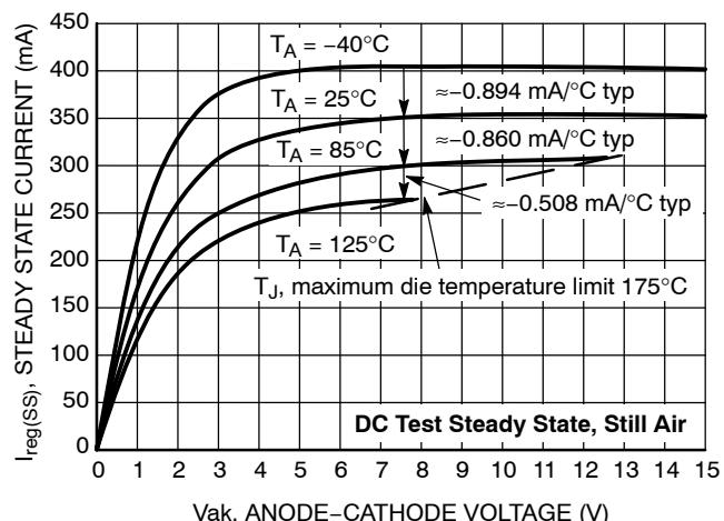
**Figure 2. Steady State Current (I<sub>reg(ss)</sub>) vs. Anode-Cathode Voltage (Vak)**
