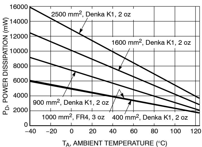
**Figure 6. Power Dissipation vs. Ambient Temperature @ T<sub>J</sub> = 175°C**
