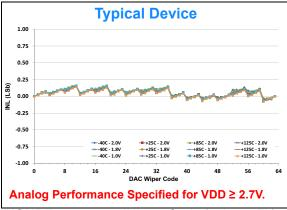
FIGURE 2-3: INL vs. Code (00h to 3Fh) and Temperature.
