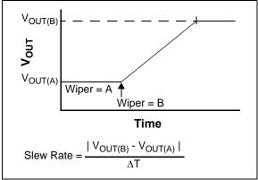
FIGURE 7-4: V<sub>OUT</sub> Pin Slew Rate.
