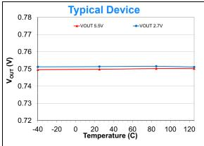
**FIGURE 2-33:**  $V_{\text{OUT}}$  Accuracy vs.  $V_{DD}$  and Temperature.
