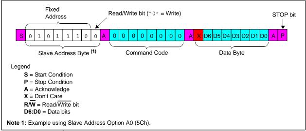
**FIGURE 5-11:** I<sup>2</sup>C Single Byte Write Command Format.
