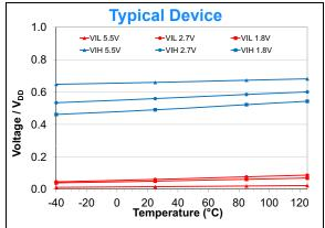
**FIGURE 2-25:**  $V_{IH} / V_{IL}$  Threshold of SDA/SCL Inputs vs. Temperature and  $V_{DD}$ .
