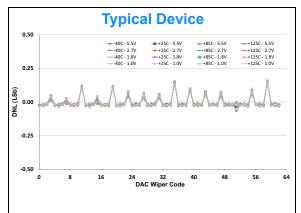
**FIGURE 2-5:** DNL vs. Code (00h to 3Fh) and Temperature.
