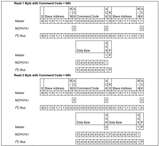
FIGURE 5-15: I<sup>2</sup>C Read Communication Behavior.
