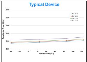
FIGURE 2-13: Zero Scale Error (ZSE) vs. Temperature.
