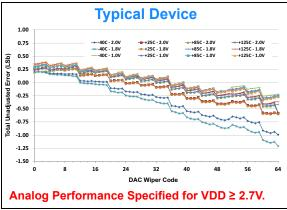
FIGURE 2-19: Total Unadjusted Error vs. Code and Temperature.
