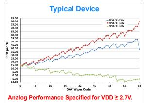
FIGURE 2-23:  $V_{OUT}$  Tempco vs. Code ( ( (  $(V_{OUT(+125C)} - V_{OUT(-40C)}) / V_{OUT(+25C,Code=FS)}) / 165$ ) \* 1,000,000),  $V_{DD} = 2.0V$ ,  $V_{REF} = 2.0V$ , 1.8V, and 1.0V.
