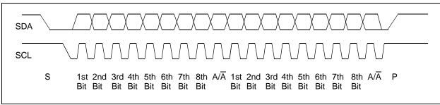
FIGURE 5-7: Typical 16-bit I<sup>2</sup>C Waveform Format.
