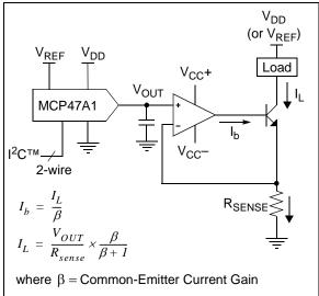
FIGURE 8-6: Digitally-Controlled Current Source.
