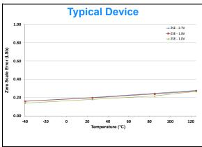
FIGURE 2-14: Zero Scale Error (ZSE) vs. Temperature.
