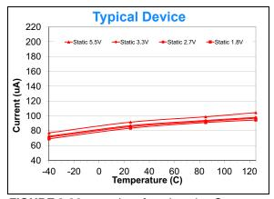
**FIGURE 2-28:** Interface Inactive Current (STATIC) vs. Temperature and  $V_{DD}$ .  $V_{DD} = 1.8V$ , 2.7V and 5.5V,  $V_{REF} = 1.0V$  and  $V_{DD}$ . (no load on  $V_{OUT}$ ,  $SCL = SDA = V_{DD}$ ).
