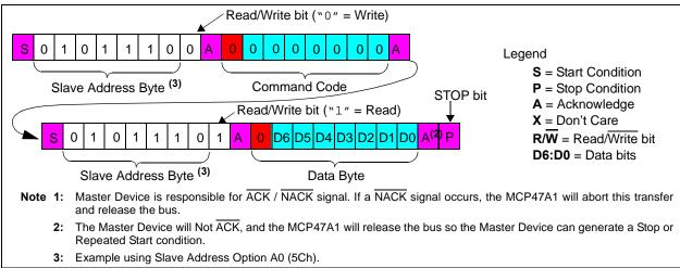
FIGURE 5-14: I<sup>2</sup>C Read Command Format.
