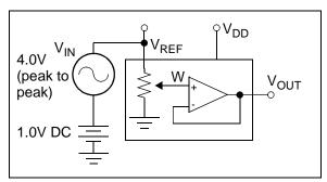
FIGURE 2-41: -3 db Gain vs. Frequency Test.
