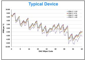
**FIGURE 2-21:**  $V_{OUT}$  Tempco vs. Code ( ( (  $(V_{OUT(+125C)} - V_{OUT(-40C)}) / V_{OUT(+25C,Code=FS)}) / 165) * 1,000,000$  ),  $V_{DD} = 5.5V$ ,  $V_{REF} = 5.5V$ , 2.7V, 1.8V, and 1.0V.
