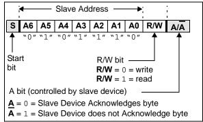
**FIGURE 5-9:** Slave Address Bits in the  $l^2$ C Control Byte.
