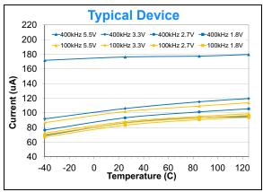
**FIGURE 2-27:** Interface Active Current  $(I_{DD})$  vs. SCL Frequency  $(f_{SCL})$  and Temperature  $V_{DD} = 1.8V$ , 2.7V and 5.5V,  $V_{REF} = 1.0V$  and  $V_{DD}$ . (no load on  $V_{OUT}$ ).
