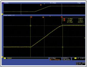
FIGURE 2-38: Half-Scale Settling Time (10h to 30h),  $V_{DD} = 5.0V$ ,  $V_{REF} = 5.0V$ ,  $R_L = 5k\Omega$ ,  $C_L = 200$  pF. (Time scale = 2  $\mu$ s / div)
