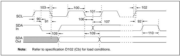
FIGURE 1-2: I<sup>2</sup>C Bus Data Timing.
