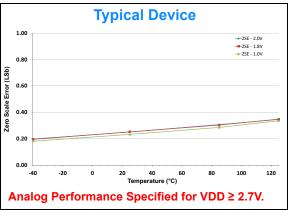
FIGURE 2-15: Zero Scale Error (ZSE) vs. Temperature.
