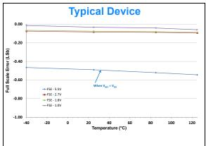
FIGURE 2-9: Full Scale Error (FSE) vs. Temperature.
