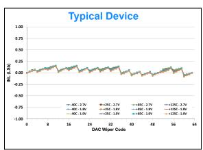
**FIGURE 2-2:** INL vs. Code (00h to 3Fh) and Temperature.
