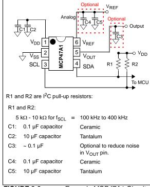
FIGURE 8-9: Example MCP47A1 Circuit.
