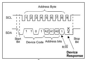
FIGURE 8-10: I<sup>2</sup>C Bus Connection Test.
