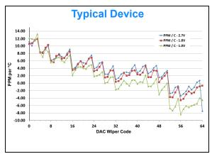
**FIGURE 2-22:**  $V_{OUT}$  Tempco vs. Code ( ( (  $(V_{OUT(+125C)} - V_{OUT(-40C)}) / V_{OUT(+25C,Code=FS)}) / 165 ) * 1,000,000 ), <math>V_{DD} = 2.7V$ ,  $V_{REF} = 2.7V$ , 1.8V, and 1.0V.
