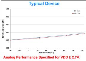
FIGURE 2-16: Zero Scale Error (ZSE) vs. Temperature.
