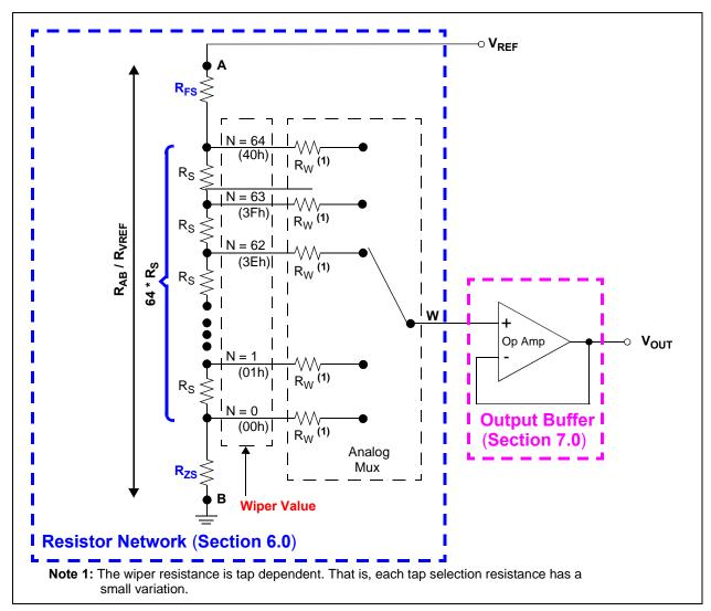
FIGURE 6-1: Resistor Network and Output Buffer Block Diagram.
