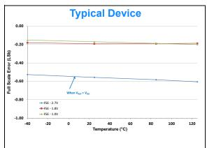
FIGURE 2-10: Full Scale Error (FSE) vs. Temperature.  $V_{DD} = 2.7V$ ,  $V_{REF} = 2.7V$ , 1.8V, and 1.0V.
