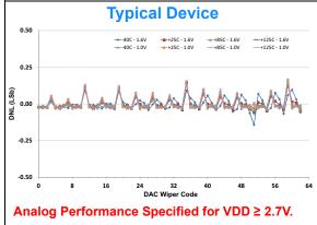
FIGURE 2-8: DNL vs. Code (00h to 3Fh) and Temperature.
