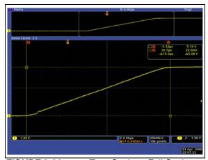
FIGURE 2-36: Zero-Scale to Full-Scale Settling Time (00h to 40h),  $V_{DD} = 5.0V$ ,  $V_{REF} = 5.0V$ ,  $R_L = 5kΩ$ ,  $C_L = 200$  pF (Time scale = 2 μs / div).
