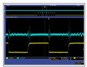
**FIGURE 2-40:** Digital Feedthrough (SCL signal coupling to  $V_{OUT}$  pin);  $V_{DD} = 5.0V$ ,  $V_{REF} = 5.0V$ ,  $F_{SCL} = 100$  kHz,  $V_{OUT} = 20h$  ( $V_{OUT}$  Voltage Scale = 20 mV/div, Time scale = 2  $\mu$ s / div).
