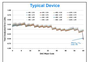
FIGURE 2-17: Total Unadjusted Error vs. Code and Temperature.
