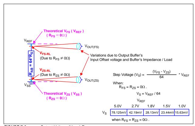
FIGURE 7-6: Output Voltage (V<sub>OUT</sub>) Error.
