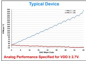
FIGURE 2-24:  $V_{OUT}$  Tempco vs. Code ( ( (  $(V_{OUT(+125C)} - V_{OUT(-40C)}) / V_{OUT(+25C,Code=FS)}) / 165) * 1,000,000$  ),  $V_{DD} = 1.8V$ ,  $V_{REF} = 1.6V$ , and 1.0V.
