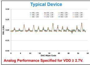
FIGURE 2-7: DNL vs. Code (00h to 3Fh) and Temperature.
