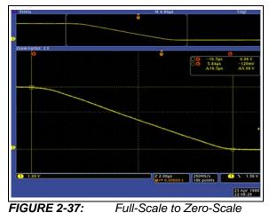
Settling Time (40h to 00h),  $V_{DD} = 5.0V$ ,  $V_{REF} = 5.0V$ ,  $R_L = 5k\Omega$ ,  $C_L = 200 pF$  (Time scale = 2  $\mu$ s / div).
