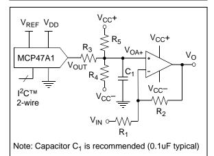
**FIGURE 8-4:** Bipolar Voltage Source with Selectable Gain and Offset Circuit.
