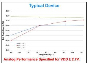
**FIGURE 2-11:** Full Scale Error (FSE) vs. Temperature.  $V_{DD} = 2.0V$ ,  $V_{REF} = 2.0V$ , 1.8V, and 1.0V.
