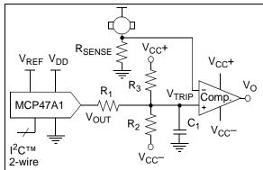
FIGURE 8-3: Single-Supply "Window" DAC.
