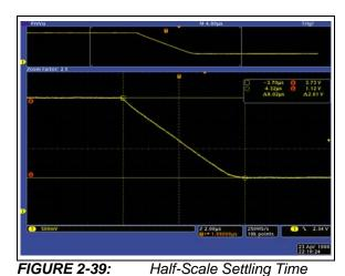
(30h to 10h),  $V_{DD} = 5.0V$ ,  $V_{REF} = 5.0V$ ,  $R_L = 5k\Omega$ ,  $C_L = 200 pF$  (Time scale = 2  $\mu$ s / div).
