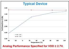
FIGURE 2-12: Full Scale Error (FSE) vs. Temperature.  $V_{DD} = 1.8V$ ,  $V_{REF} = 1.6V$ , and 1.0V.
