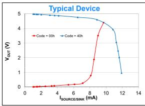
**FIGURE 2-31:**  $V_{OUT}$  vs. Source / Sink Current.  $V_{DD} = 5.0V$ .
