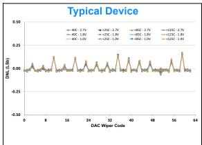
FIGURE 2-6: DNL vs. Code (00h to 3Fh) and Temperature.
