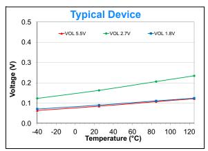
**FIGURE 2-26:**  $V_{OL}$  (SDA) vs.  $V_{DD}$  and Temperature.
