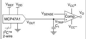
FIGURE 8-1: Set Point or Threshold Calibration.
