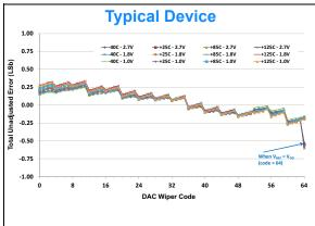
FIGURE 2-18: Total Unadjusted Error vs. Code and Temperature.
