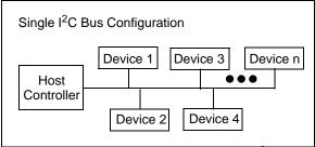
**FIGURE 5-1:** Typical Application PC Bus Configurations.
