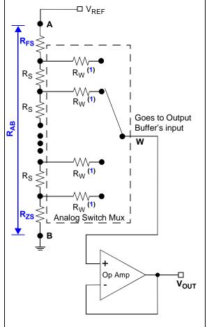
**Note 1:** The wiper resistance is tap dependent. That is, each tap selection resistance has a small variation.
