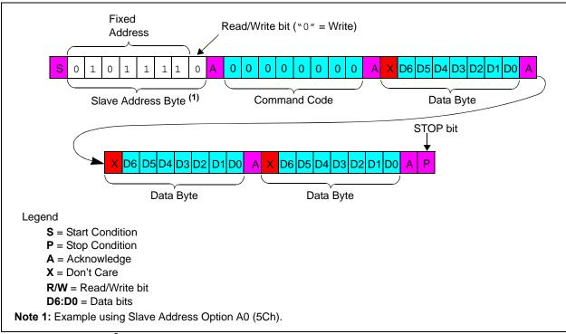
**FIGURE 5-12:**  $l^2C$  Write Command Format.
