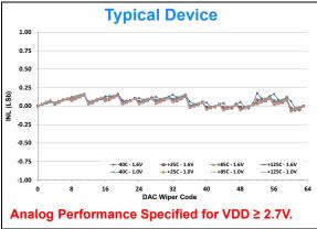
FIGURE 2-4: INL vs. Code (00h to 3Fh) and Temperature.
