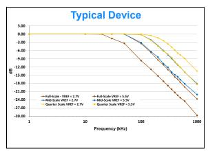
**FIGURE 2-35:** -3dB Bandwidth vs Frequency,  $V_{DD} = 5.5V$ .
