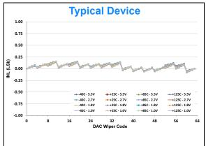
**FIGURE 2-1:** INL vs. Code (00h to 3Fh) and Temperature.
