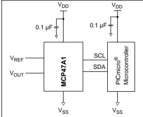
FIGURE 8-8: Typical Microcontroller Connections.
