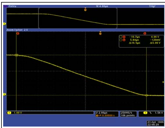
FIGURE 2-37: Full-Scale to Zero-Scale Settling Time (40h to 00h), V_{DD} = 5.0\text{V} , V_{REF} = 5.0\text{V} , R_L = 5\text{k}\Omega , C_L = 200\text{pF} (Time scale = 2\text{ }\mu\text{s} / \text{div} ).
