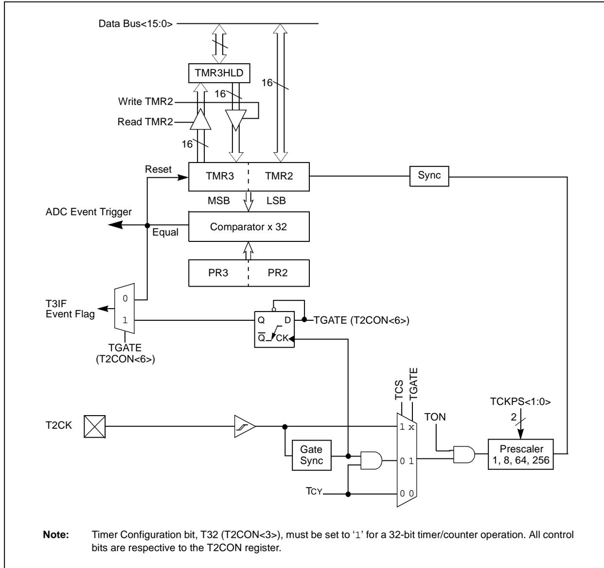
**FIGURE 10-2: 16-BIT TIMER2 BLOCK DIAGRAM**
