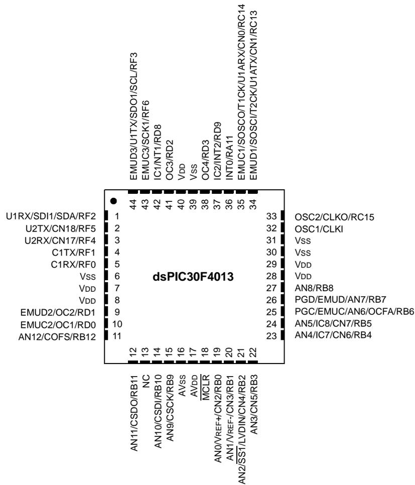
**Note 1:** The metal plane at the bottom of the device is not connected to any pins and is recommended to be connected to Vss externally.
