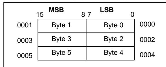
All byte loads into any W register are loaded into the LSB. The MSB is not modified.
