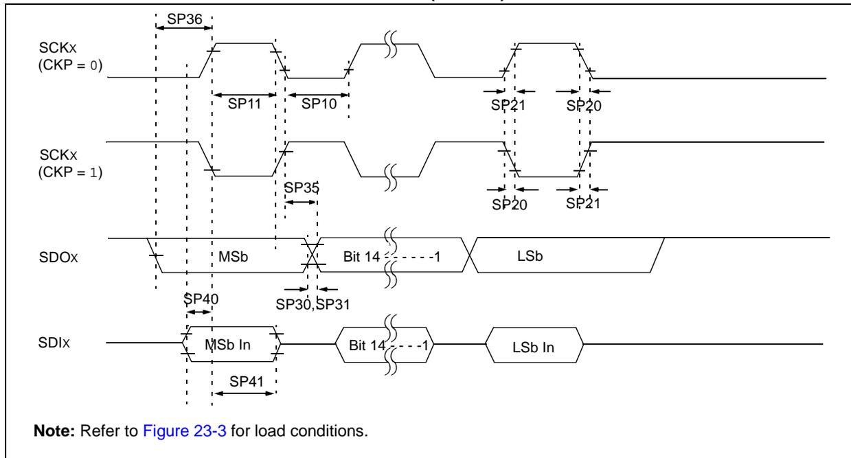
**TABLE 23-31: SPI MODULE MASTER MODE (CKE = 1) TIMING REQUIREMENTS**
