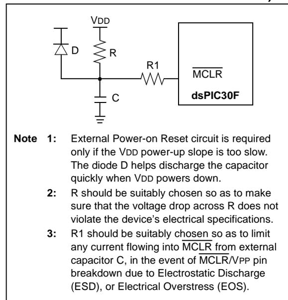
**Note:** Dedicated supervisory devices, such as the MCP1XX and MCP8XX, may also be used as an external Power-on Reset circuit.
