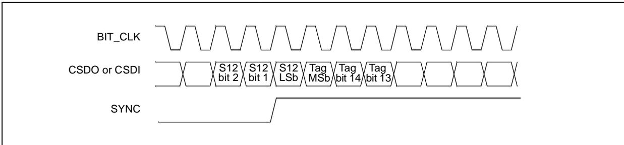
**FIGURE 18-4: I<sup>2</sup>S INTERFACE FRAME SYNC TIMING**
