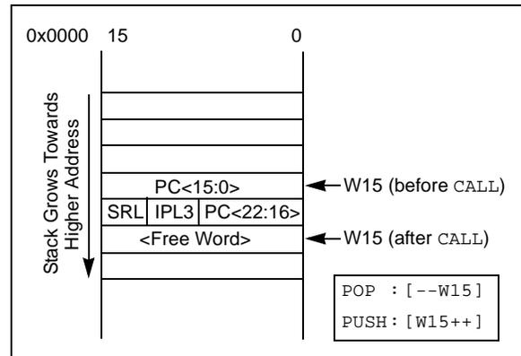
**Note 1:** The user can always lower the priority level by writing a new value into SR. The Interrupt Service Routine must clear the interrupt flag bits in the IFSx register before lowering the processor interrupt priority, in order to avoid recursive interrupts.
