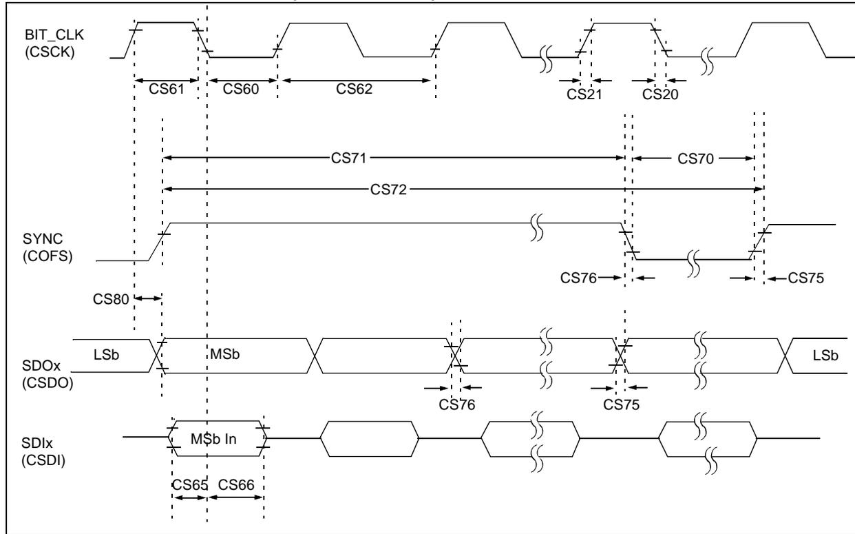
**TABLE 23-29: DCI MODULE (AC-LINK MODE) TIMING REQUIREMENTS**
