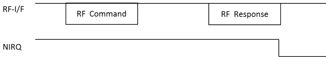
Figure 6-3 RF transmission complete interrupt
