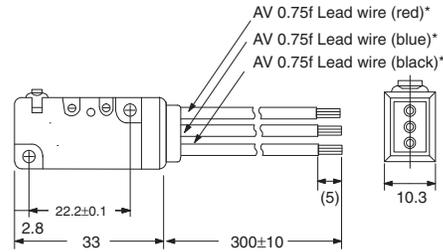
\* UL/CSA approved models have AWG20 UL approved wiring.
