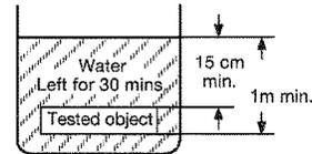
**Note:** The object to be tested is left in the water for 30 minutes on condition that the distance between the surface of the water and the top of the object be 15 cm minimum and the distance between the surface of the water and the bottom of the object be 1 m minimum.
