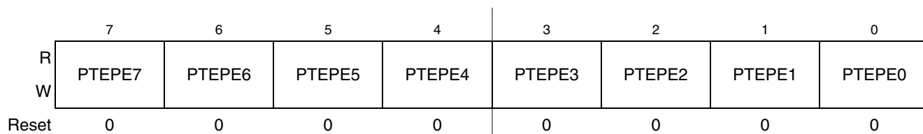
Figure 6-24. Internal Pullup Enable for Port E (PTEPE)
