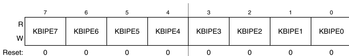
Figure 9-4. KBI Pin Enable Register
