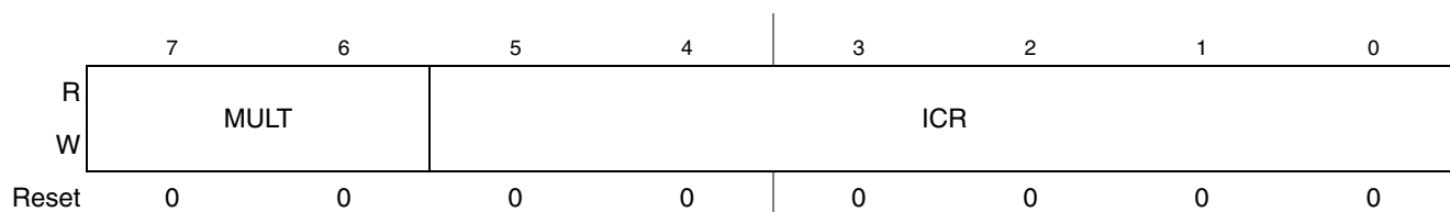
Figure 11-4. IIC Frequency Divider Register (IICF)
