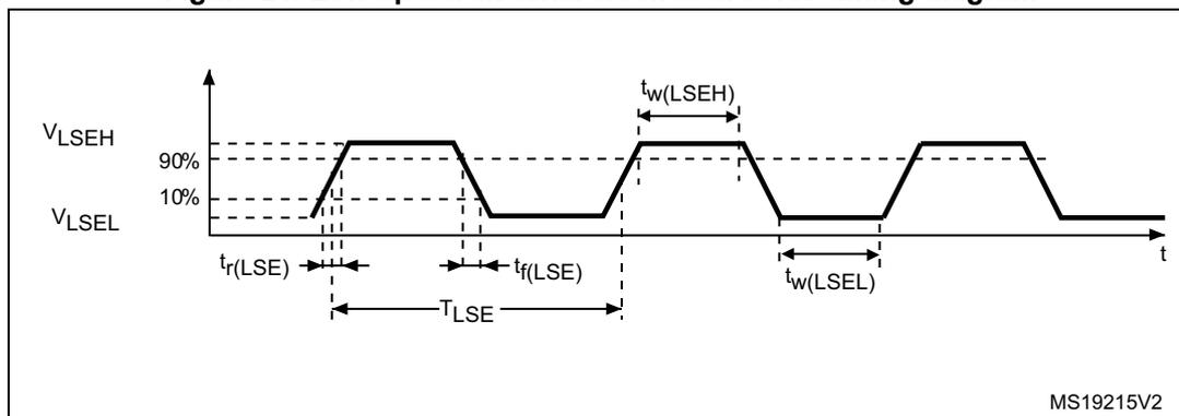
Table 55. Low-speed external user clock characteristics<sup>(1)</sup> – Bypass mode
