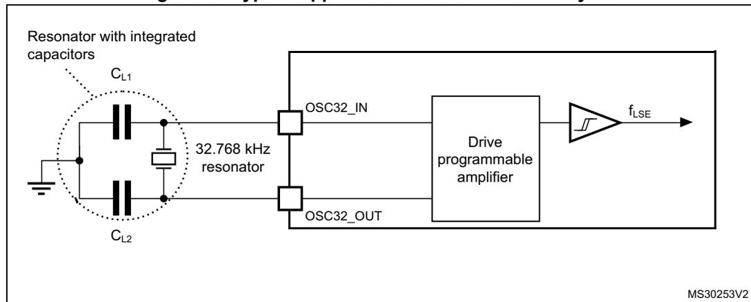
Note: No external resistors are required between OSC32\_IN and OSC32\_OUT, and it is forbidden to add one.
