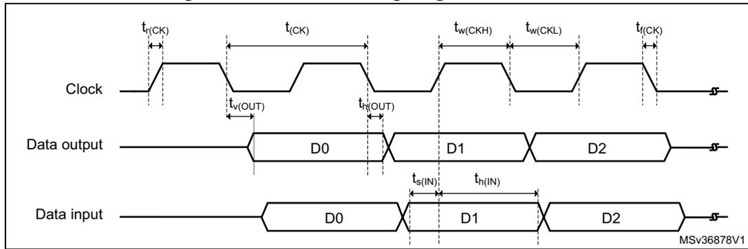
Figure 33. Quad-SPI timing diagram - DDR mode
