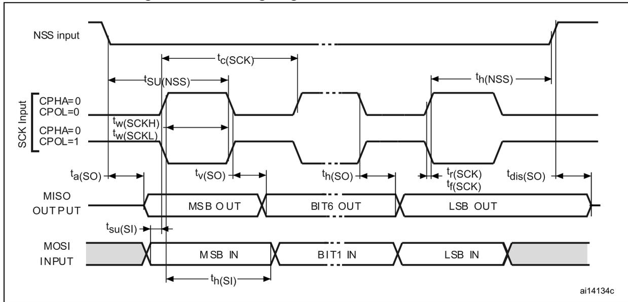
Figure 30. SPI timing diagram - slave mode and CPHA = 1
