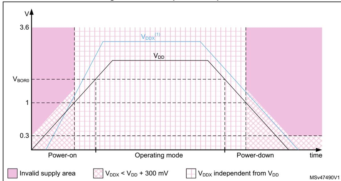
1.  $V_{DDX}$  refers to any power supply among  $V_{DDA}$ ,  $V_{DDUSB}$ ,  $V_{LCD}$ .
