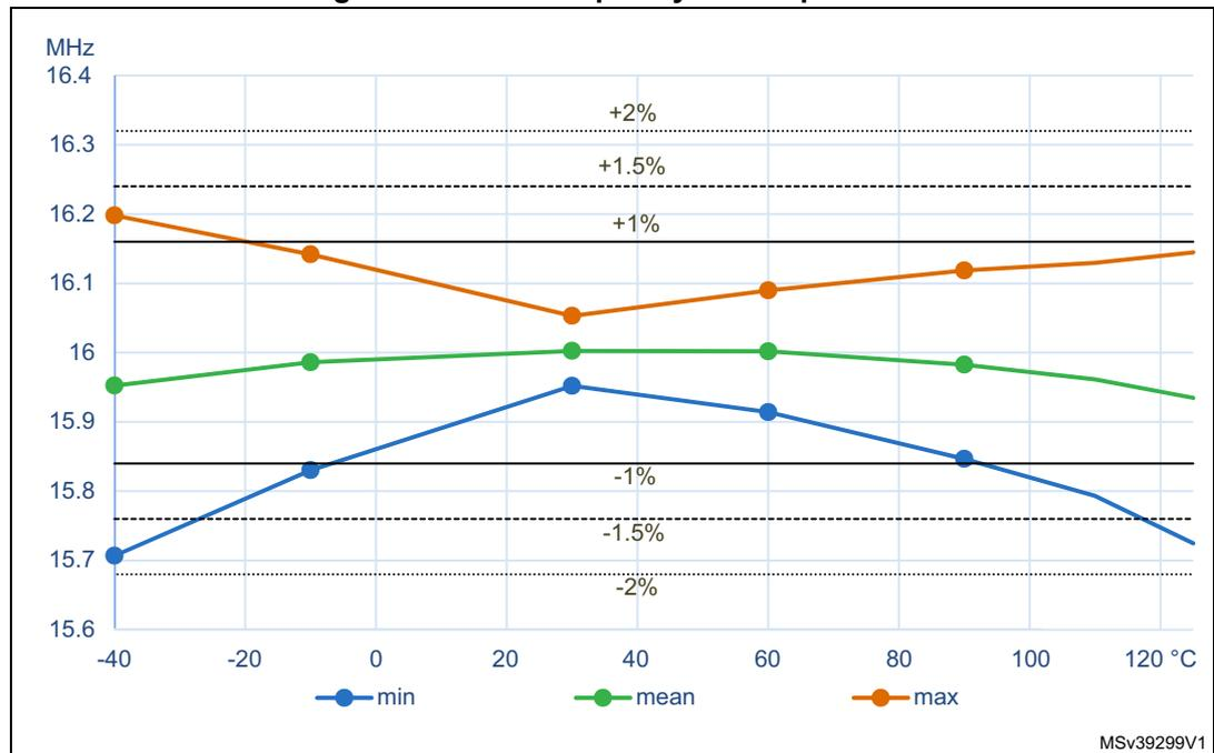
Multi-speed internal (MSI) RC oscillator
