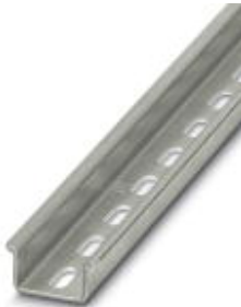
DIN rail, material: steel galvanized and passivated with a thick layer, perforated, height 15 mm, width 35 mm, length: 2000 mm
