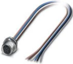
Sensor/actuator flush-type socket, 6-pos., M8, rear/screw mounting with M10 fastening thread, with 0.5 m TPE litz wire, 6 x 0.14 mm<sup>2</sup>
