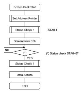
Note: This command is available when hardware column number and software column number are the same. Hardware column number is related to MD2 and MD3 setting. Software column number is related to Set Text Area and Set Graphic Area command.
